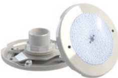
LED lamp Moonlight PLW300 12 V / 15 W white, luminous flux 1250 lm
